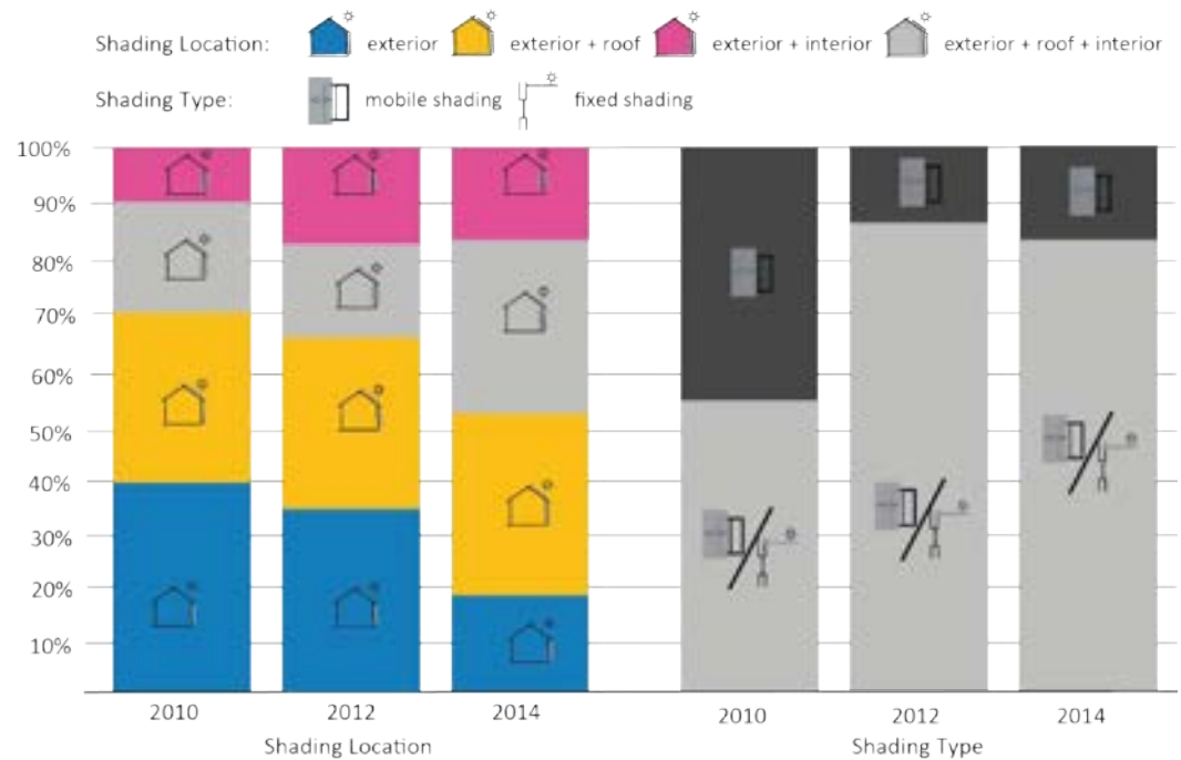
Figure 1.20: Distribution of external, internal, fixed and moveable sun protection devices presented by the SDE houses. Source: University of Wuppertal, Susanne Hendel
